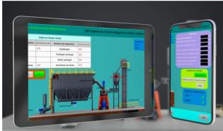
4. Automatically and evenly adjust the feeding amount of raw material according to the current of the main mill and fan to achieve the highest grinding efficiency.
